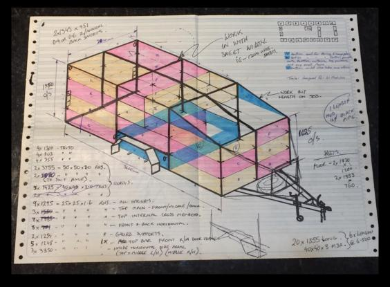
The design would carry all modules, lighting gear, carpet curtains, controllers and panels, seats, repair tools and any incidental hardware Spare wheel and jack.
