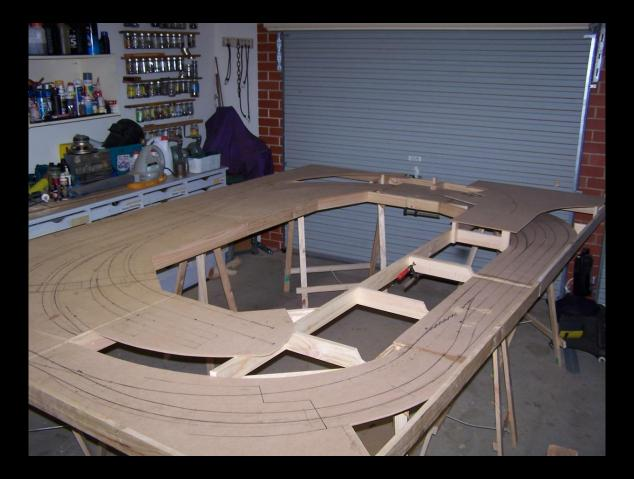
Timber construction with 6mm MDF baseboard The frames are combination 70 x 19 & 45 x 19mm Pine.
