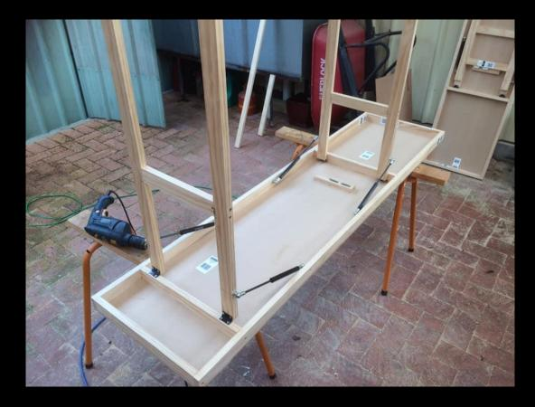
Support legs made using Pine and hinges. Each leg assembly is made to fit INTO the baseboard or fit FLUSH with the framework.
